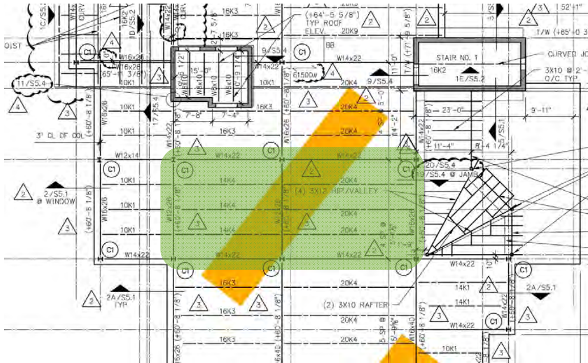
[Figure 33. Portion of the Solar Array Layout overlaid on the Structural Roof Drawing]
